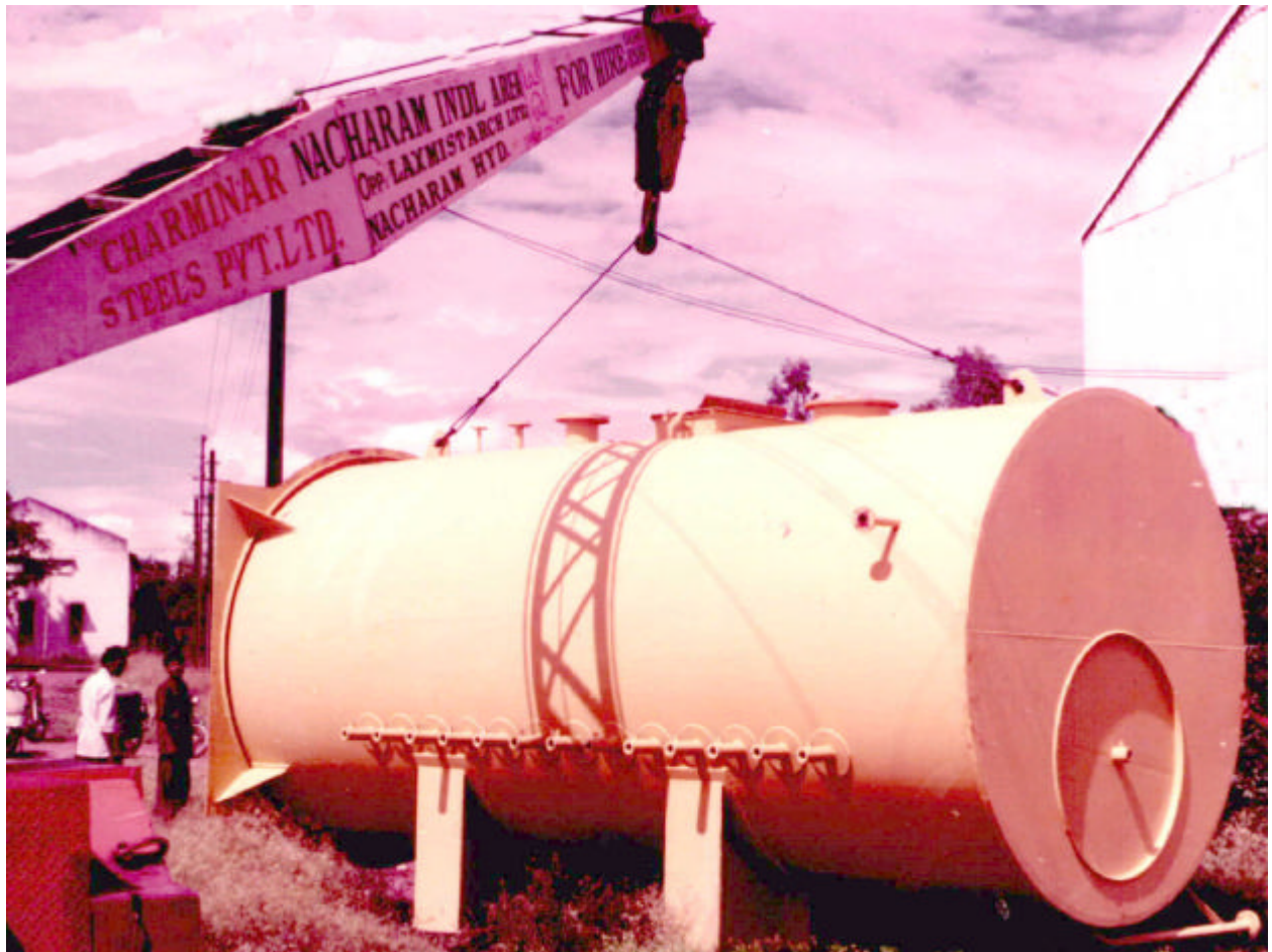
Sugar Mill Fabricated Tank under shipment from works. SS Fabricated tank for dairy plant under Installation in Tanzania.
