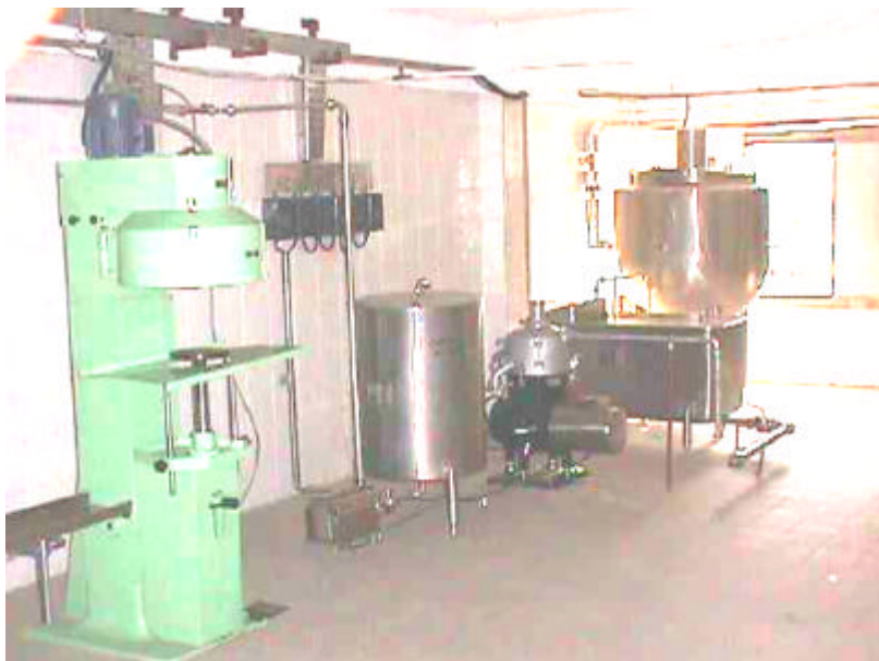
Ghee Vat, Settling Tank, Clarifier & Clarified Ghee Tank
